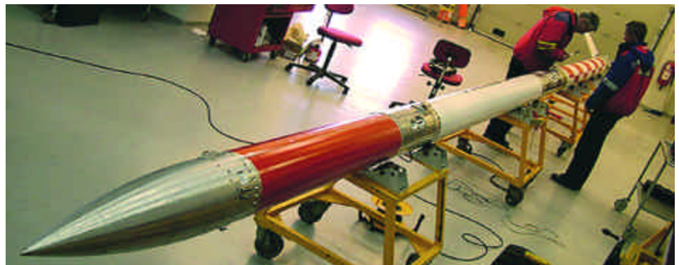
Technicians finalize the assembly of the pencil-like Hybrid Sounding Rocket.
