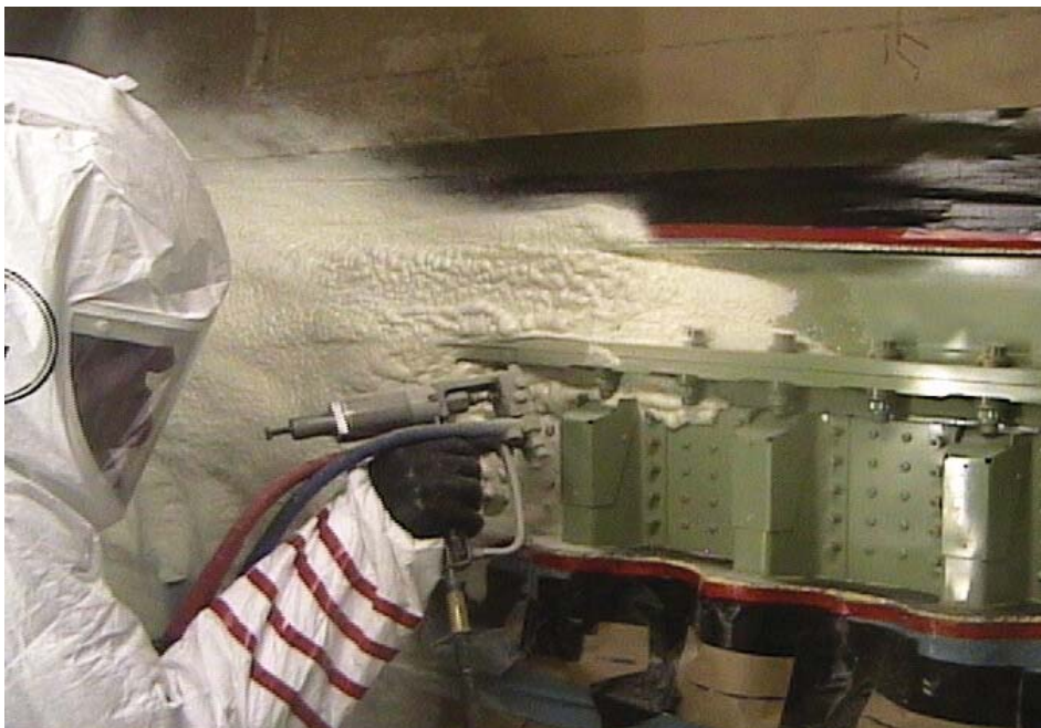
As one of a three-sprayer team, technician James Duke applies foam to the ET-131 Liquid Oxygen / Intertank flange.
