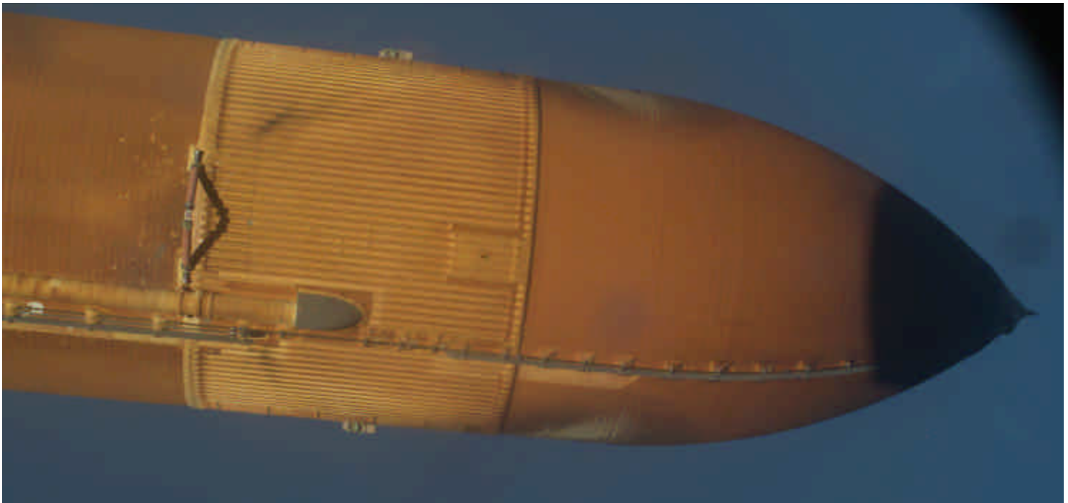
ET-119 shown with relatively minor foam loss after separation from Discovery.
