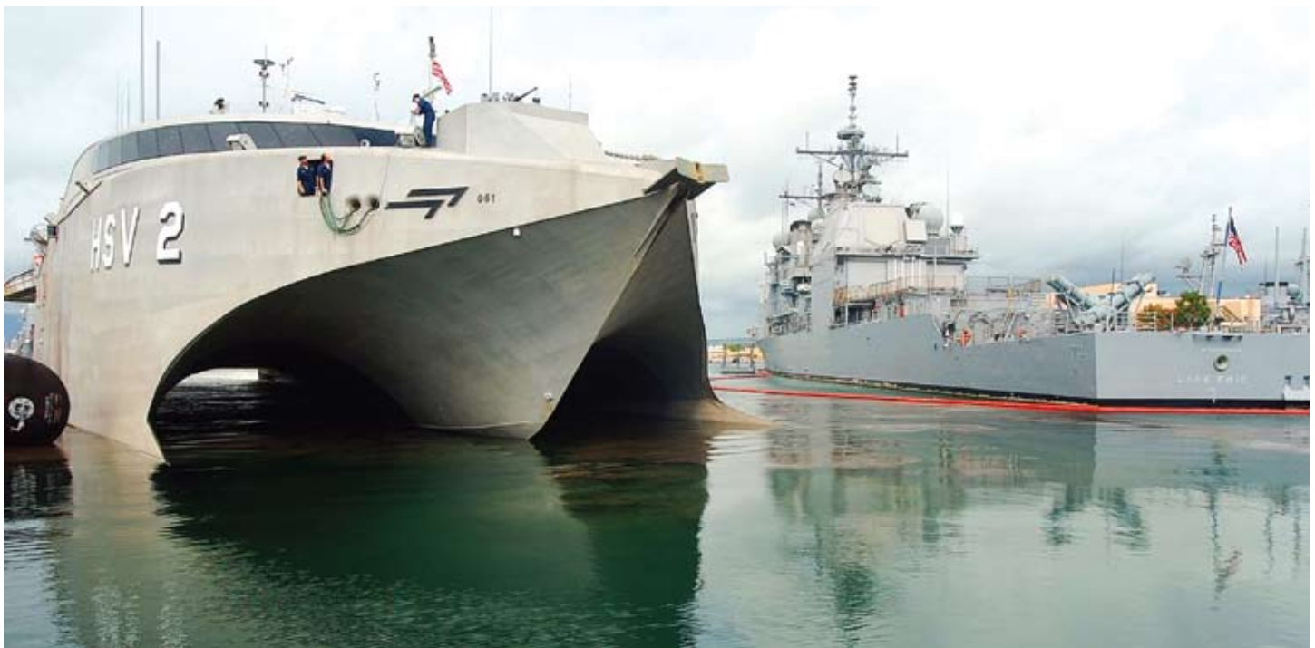
The Joint High Speed Vessel (JHSV) program is a high-speed, shallow-draft vessel intended for rapid transport of medium-sized cargo payloads. JHSV will reach speeds of 35-45 knots and allow for fast transit and deployment of conventional or special forces as well as equipment and supplies. The JHSV will be able to transport Army and Marine Corps units with their vehicles, or reconfigure to carry troops for an infantry battalion.
