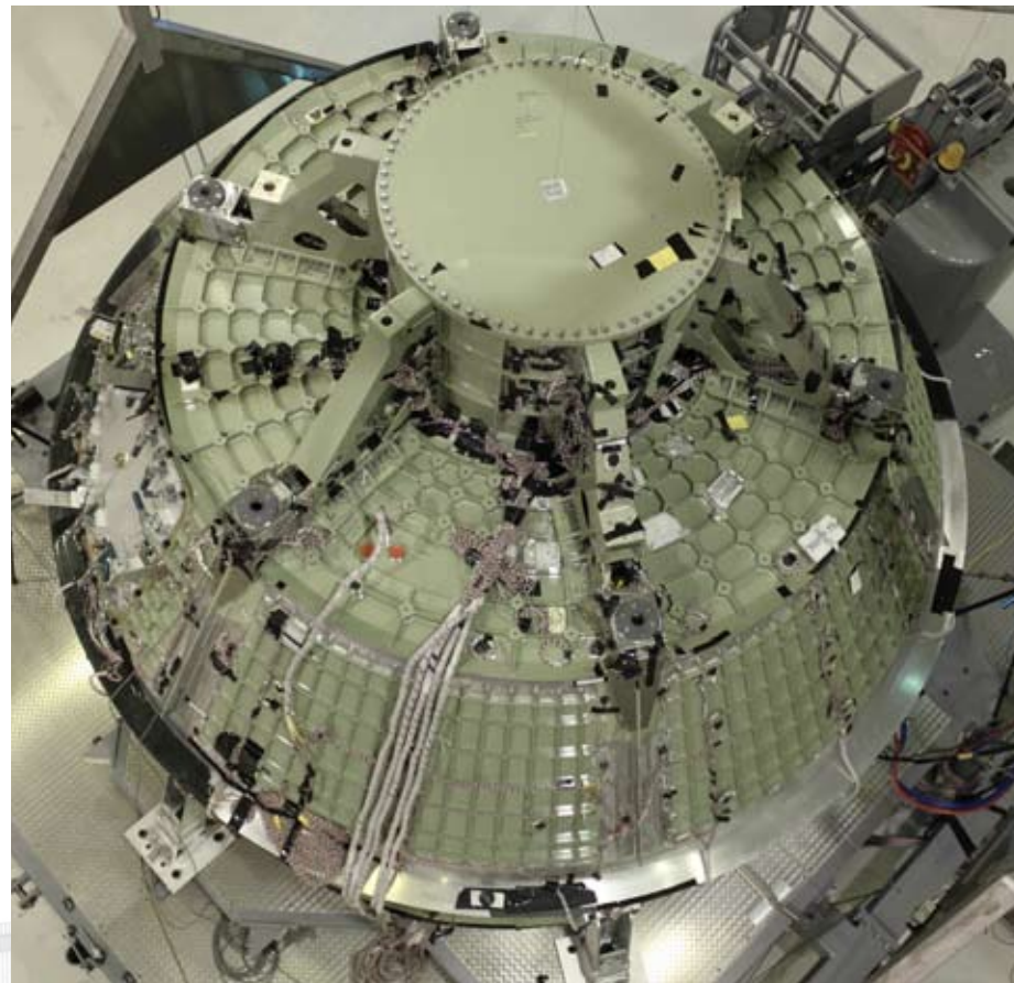
Lockheed Martin's Orion Crew Module Ground Test Article recently underwent a successful structural proof pressure test at Michoud.
