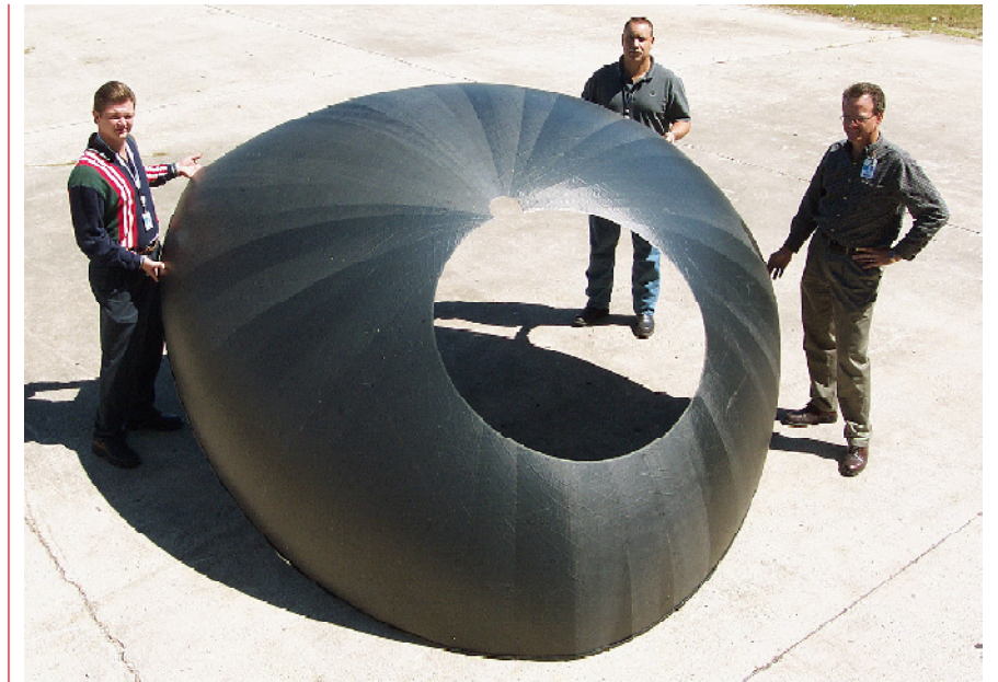
Fiber Placement Machine sample dome arrives from Ingersoll Bobby Biggs (from left), Wayne Richmond and Barry Keegan display a ten-foot wide graphite-epoxy dome recently fabricated on the new Fiber Placement Machine. Weighing only 23 pounds, the dome is a sample part fabricated during machine checkout last month. The Fiber Placement Machine is a critical piece of equipment for the National Center for Advanced Manufacturing at Michoud. Shipments of machine parts are currently arriving, and operation is targeted for February 2002.
