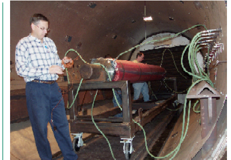
Inside the autoclave, Bill Frey (left) fastens sensors to the composite strut as it is prepared for the curing process.
