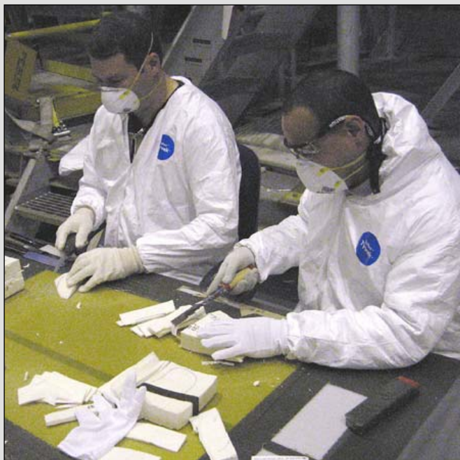
Thermal Protection Systems technicians Ronnie Clark and Carlos Saavedra dissect a recently sprayed PAL ramp mock-up panel.
